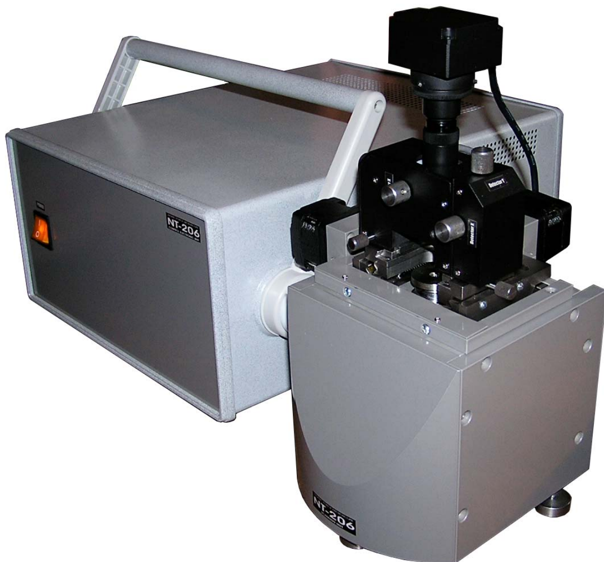
Fig. 1.1. General view of atomic force microscope NT-206 in basic configuration: scanning unit (foreground device) with control electronic unit (background device).
